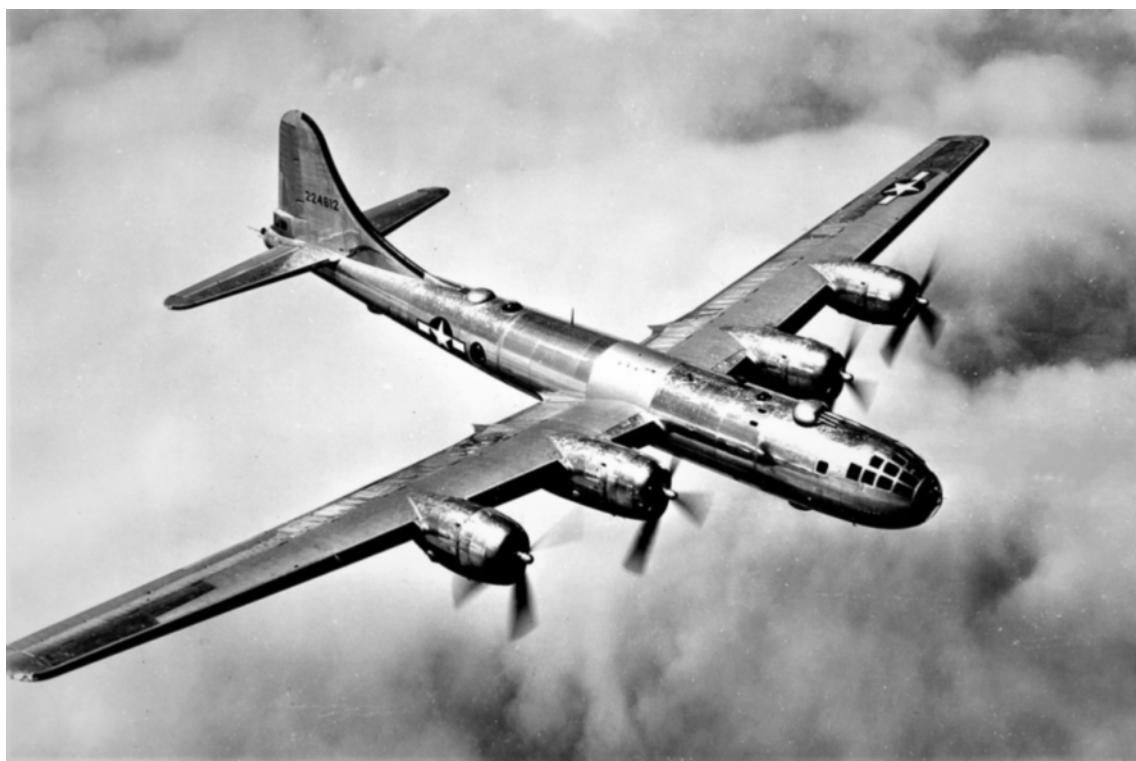
Boeing B-29 Superfortress in flight – U.S. Air Force, Public domain, Wikimedia. The B-29 Superfortress, a four-engine propeller-driven heavy bomber designed for high-altitude bombing and low-altitude night incendiary bombing, was the most expensive program of World War Two. The B-29 state-of-the-art technology with a pressurized cabin and an analog computer-controlled fire control system allowing one gunner and a fire control officer to control four remote machine gun turrets, made it effective throughout the Korean War and was not retired until the 1960s after 3,970 had been built.
