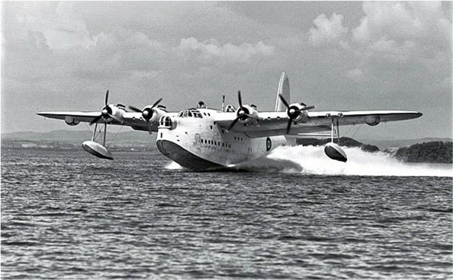
Short Sunderland Mark IIIA with Mark V radar blisters and nose guns – Unknown author, Canadian Air Force, Public domain, Wikimedia
